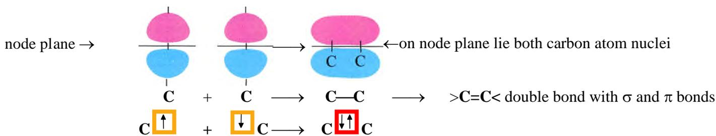
4. Figure. C and C atomic orbitals fuse into  $\pi$  molecular orbital and form in double bond  $>\text{C}=\text{C}<$  second bond after sigma  $\sigma$  bond C—C formation. On common node plane lie both carbon atomic nuclei, but negative charge (—) density between positive charged atom nuclei weakened repulsion forces and strengthening covalent bond together with sigma bond  $\sigma$  on formed double bond  $>\text{C}=\text{C}<$ .
