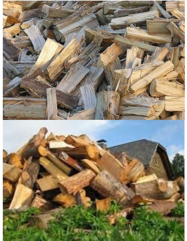
14 Fig. To split firewood can easy on fiber direction of cellulose and hardly never perpendicular of cellulose fiber direction.
